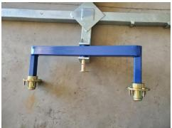
5.) Use 13mm nut and bolt to hold pin to tab, tighten.
