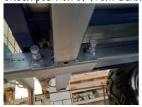
23.) Find crane and winch mount, 2 long bolts and nuts, hold upper section on lining up holes, install 2 bolts and tighten nuts.
