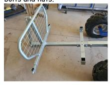
16.) Install outriggers and retaining handles.
