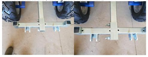
13.) Find front bunk frame and slide onto the frame.
