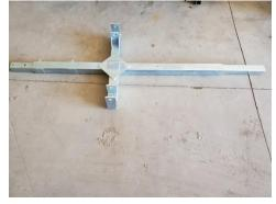
4.) Place the walking beams between the tabs on either side, there is not a right or left, either walking beam can be used for both sides and insert pins.
