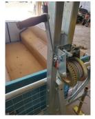
26.) Remove bolt and reverse the position of the swivel lock pin.
