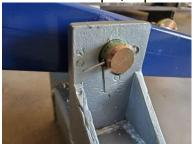
7.) Grease both pins liberally using a grease gun.
