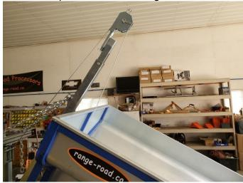
Loosen 4 main frame bolts and pull inner tube forward or backward to make frame length shorter or longer.
