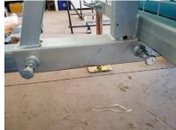
Check position of front bunk mount and tighten bolts. 21.)
