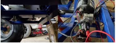
16.) Install hydraulic hose, mount to pump and cylinder, use tabs on frame to hold the hose.
