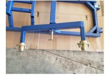
4.) Install 13mm bolt & nut washer through the plate on the pin and and the frame tab, tighten nut & Bolt. Install cotter pin, repeat for the opposite side.
