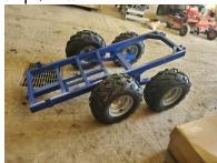
8.) Install frame tube into main frame, holes at coupler end face up & down.
