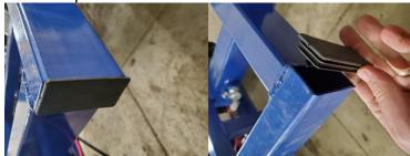
24.) Mount 2 reflectors on mounts at rear of tub.
