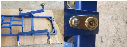
6.) Install all 4 tires and tighten wheel nuts to 40ft/lbs.
