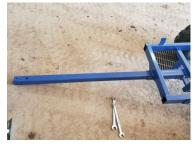
9.) Large bolt goes through frame tube and main frame, tighten nut. Tighten 2 bolts on the side of the frame rail, then tighten retaining nuts.
