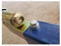
13.) Slide tongue jack to desired position, usually about 15cm (6") back of 1st swivel coupler bolt.
