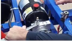
5) When oil starts to seep out of the threads, stop turning until there is no pressure left in the oil coming out, usually just a few seconds.
