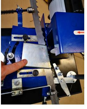
Install compressor handle and compressor support on top of press plate
