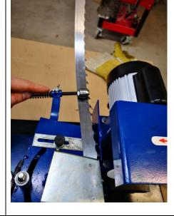
Slide the Right pressure wheel over the center of the blade
