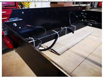
You can now tighten all the wire harness brackets to hold the wire harness snugly in place
