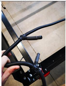
Photo of the connectors securely attached to the lights
