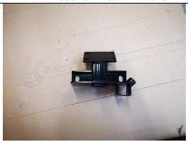
This photo shows the axle cross piece and the fender brackets installed
