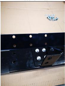
Once all the bolts are installed loosely, Use a tool to line up the ends
