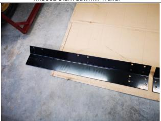
There must be a small square hole on the left end of the frame piece for mounting a marker light later
