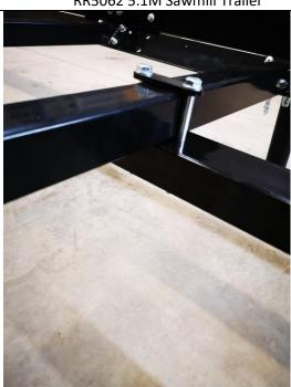
The front cross piece is secured to the draw bar using the longer black bracket
