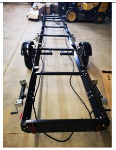
Now you will need the wiring harness brackets, hardware and zip-ties to secure the wiring harness
