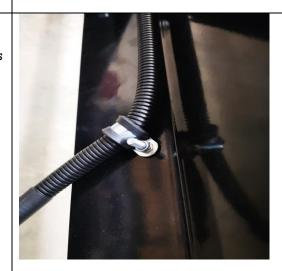
Move on up to the front of the trailer and simply wrap the 4-pin connector around the draw bar so it does not drag on the ground and is out of the way until needed
