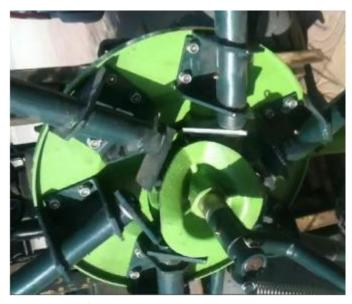
B.Assemble of the wheel (1)open the B-pin and spacer
