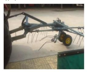
(4) fix the lock pin in the lowest hole
