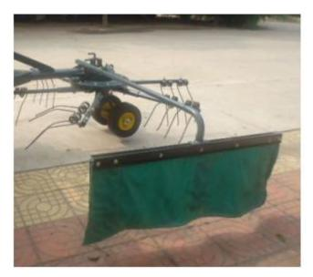
Adjusting the length of grass guard by fix the pin in different holes of rod and sleeve.(remark: the length have to be longer than the spring teeth reach)
