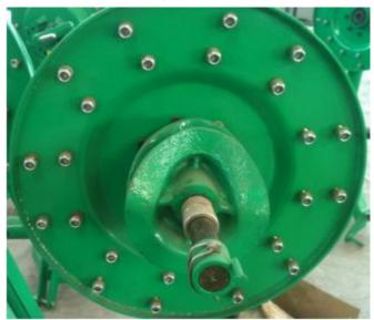
(3) fix the bearings into the track and tighten the arm on the rotary disc one by one by the nuts.
