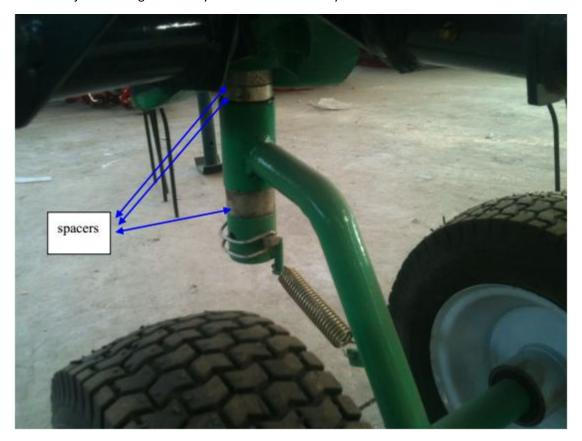
Fix the spacers previous than wheel sleeve, the working height is higher Fix the spacers below the wheel sleeve, the working height is lower 5 storage
