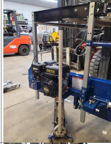
Attach push handle to the post on the lower two of the four holes.
