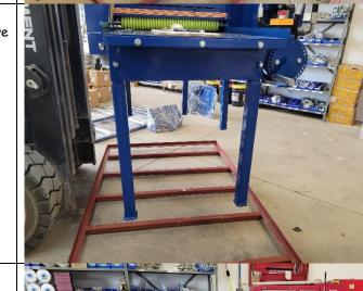
After these legs are attached the machine can be lowered and set on the ground
