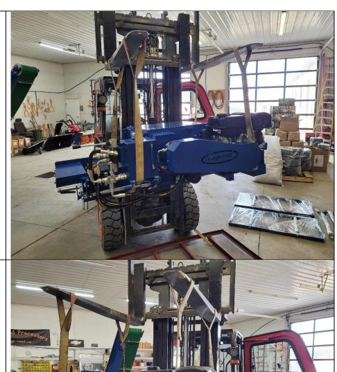
Straps need to be placed on the outside of the engine and hydraulic tank as shown in pictures
