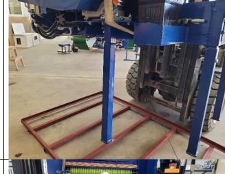
Attach the remaining two square bottom legs to entrance side (control side) of machine
