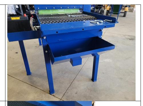
Locate the four collared bolts on the bottom of the main body
